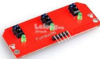
Figure 3.7: The line sensor module [10]
