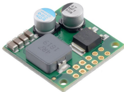
Figure 11 12V, 4.5A Step-Down Voltage Regulator
