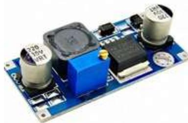
**Figure 12 LM2596 step-down switching regulator**
