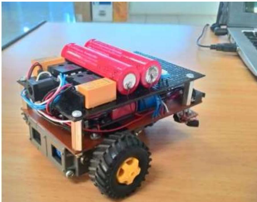
**Figure 4 an obstacle avoiding robot**
