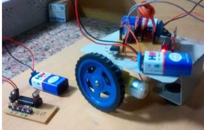
**Figure 6 Radio Frequency (RF) Controlled Wireless Robot**
